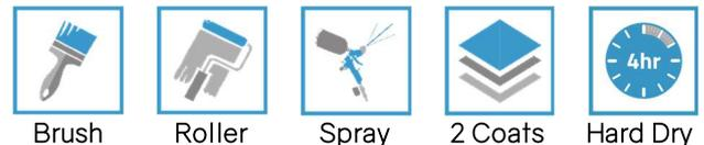
Black Dog is ready for use and should not be thinned. Stir thoroughly before use. Apply by brush, roller or spray. A minimum of two coats of should be applied. The first coat should be allowed to dry (normally 2-4 hours depending on weather conditions) before the second coat is applied. Concrete and some stone surfaces may be porous so an initial primer coat should be applied.
