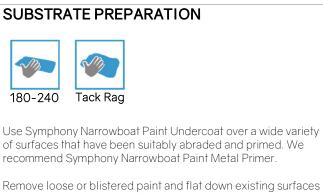
Remove loose or blistered paint and flat down existing surfaces with 180-240 Grit sanding. Remove sanding dust by wiping with a tack cloth. All surfaces must be sound, clean, dry and free from dust, grease or any other surface contaminants before application.
